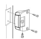
Close the door and using the lock case as a guide mark the position of the remaining component - the 'staple' - on the door frame. Chisel out a recess in the door frame to hold the staple flush with the frame and fix it with the screws provided.
