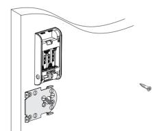
Fix screw to completely secure battery pack.
